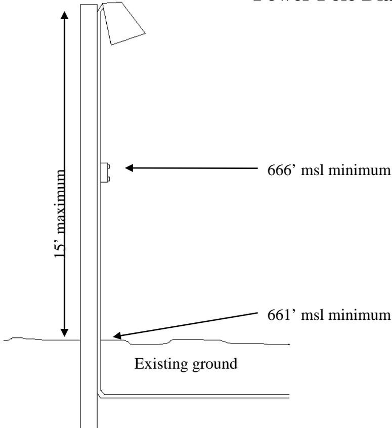
Installation must meet or exceed National Electric Code standard for wet locations and any additional requirements set by the Corps of Engineers as listed below.
